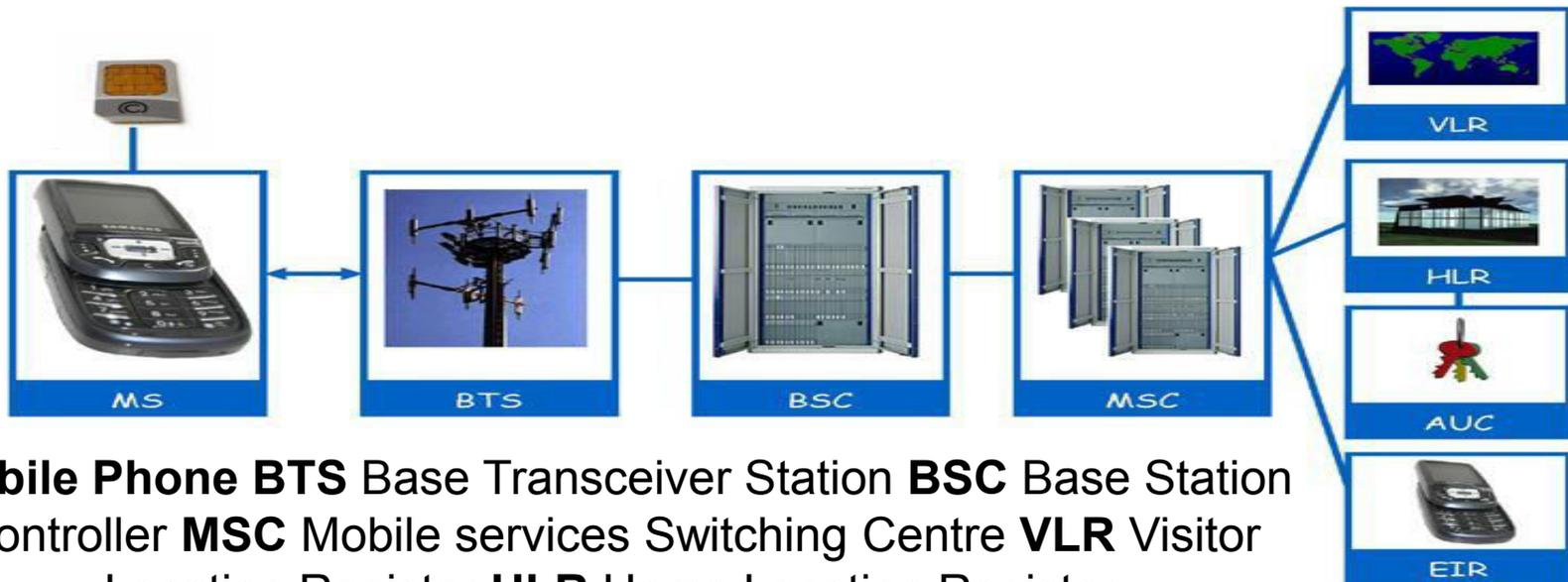
**Mobile Phone** **BTS** Base Transceiver Station **BSC** Base Station Controller **MSC** Mobile services Switching Centre **VLR** Visitor Location Register **HLR** Home Location Register
