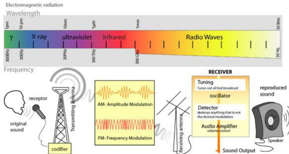
In AM amplitude changes but frequency does not. AM frequencies range from 540,000 Hz to 1,600,000 Hz usually listed in kHz.
